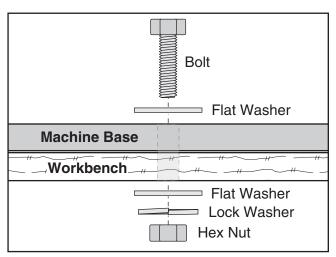
Figure 5. Example of a "Through Mount" setup.
